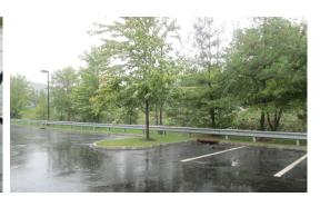
This site is located on Amboy Avenue. The site uses traditional catch basins to capture its parking lot runoff. However, with nearby existing swales, the site could benefit from creating curb cuts that direct stormwater into the swales or additional rain garden plantings. In addition, the current state of the asphalt has deteriorated enough to justify its replacement. The site could benefit from porous asphalt as it will promote water infiltration and reduce puddling.
